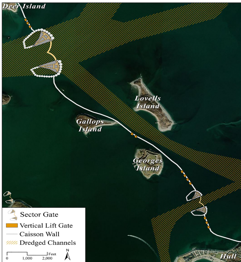
Fig. 2 Outer harbor barrier configuration. (1 ft = 0.3048 m). From Kirshen et al. (2018)
